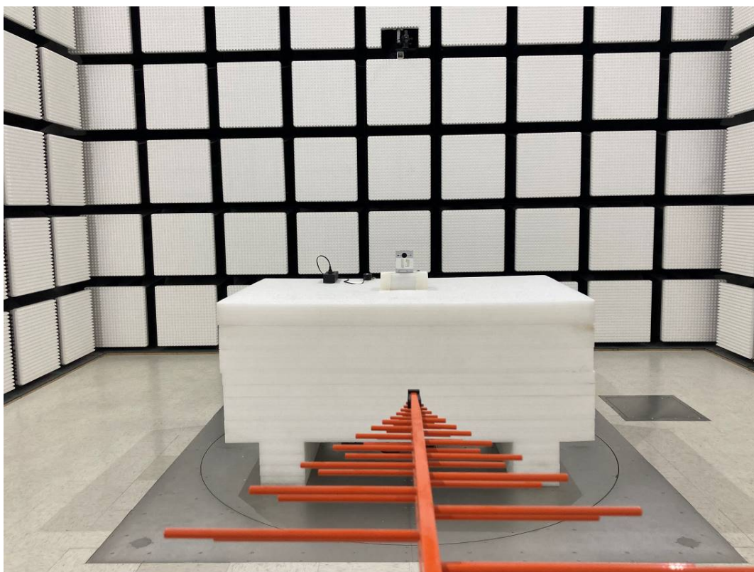
Radiated Emission 30M-1GHz View POE
