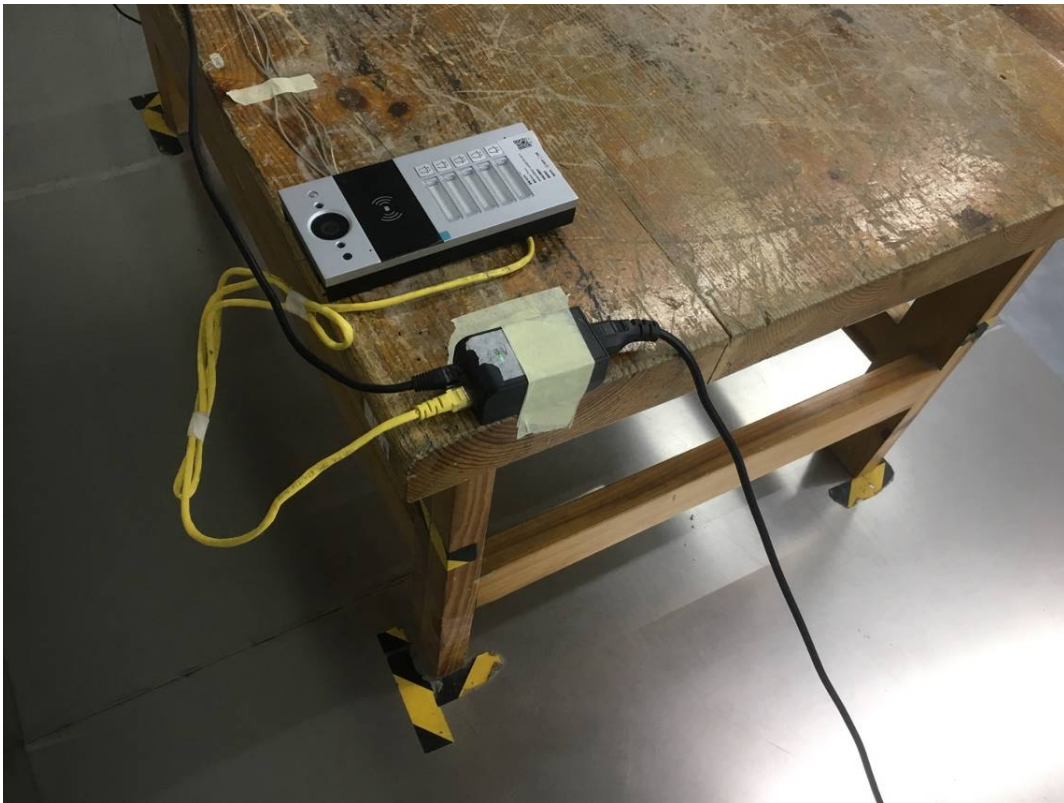
Conducted Emissions Side View POE
