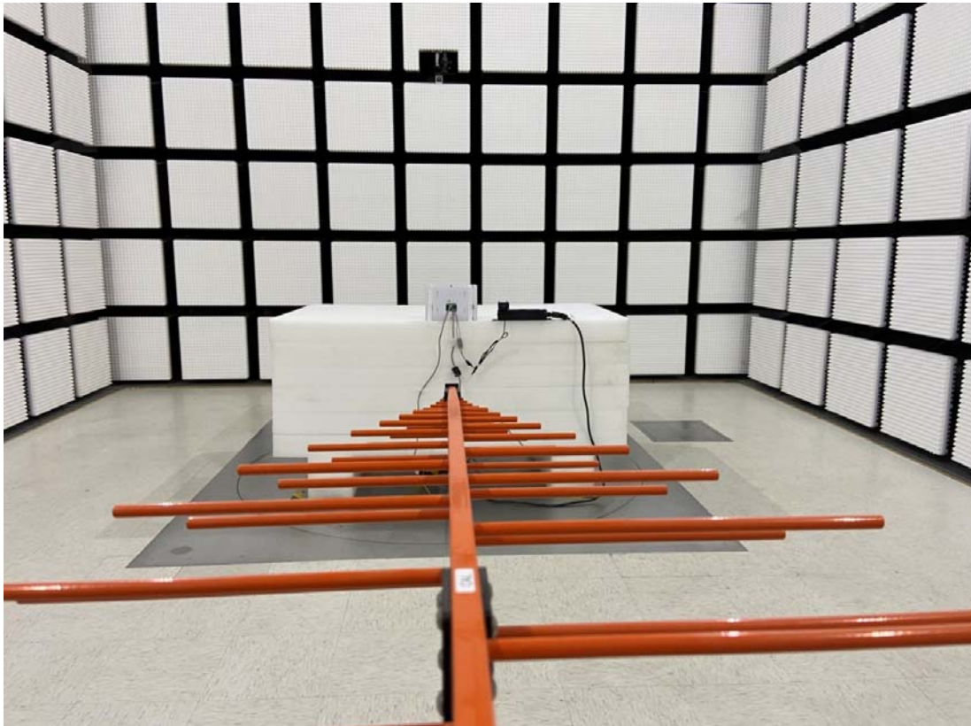
Radiated Emission Below 1G rear View - AC/DC Adapter
