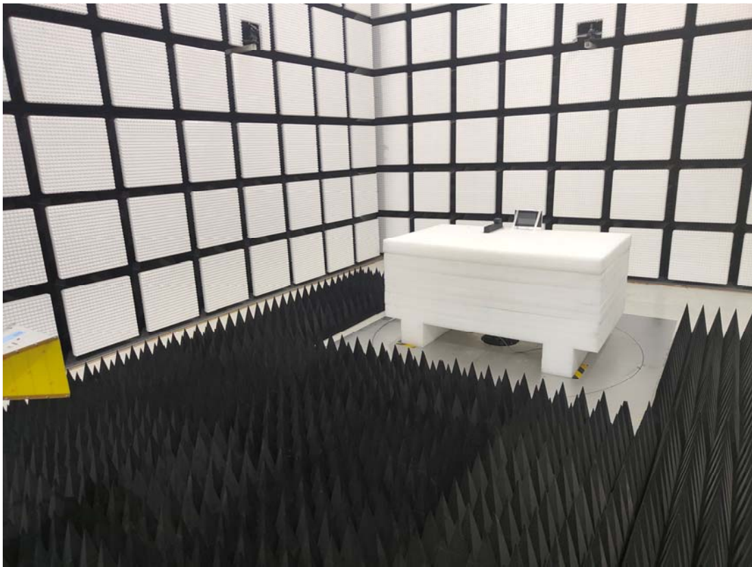
Radiated Emission Above 1G rear View-AC/DC Adapter
