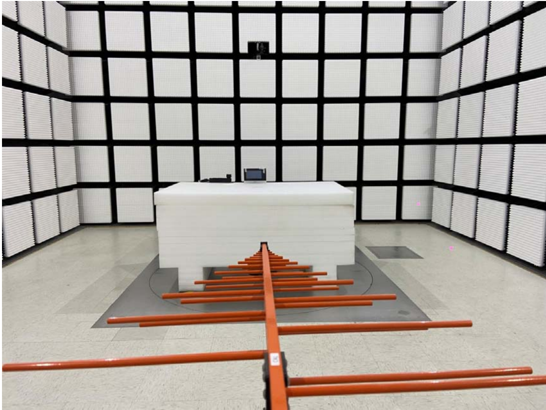
Radiated Emission Below 1G rear View - AC/DC Adapter
