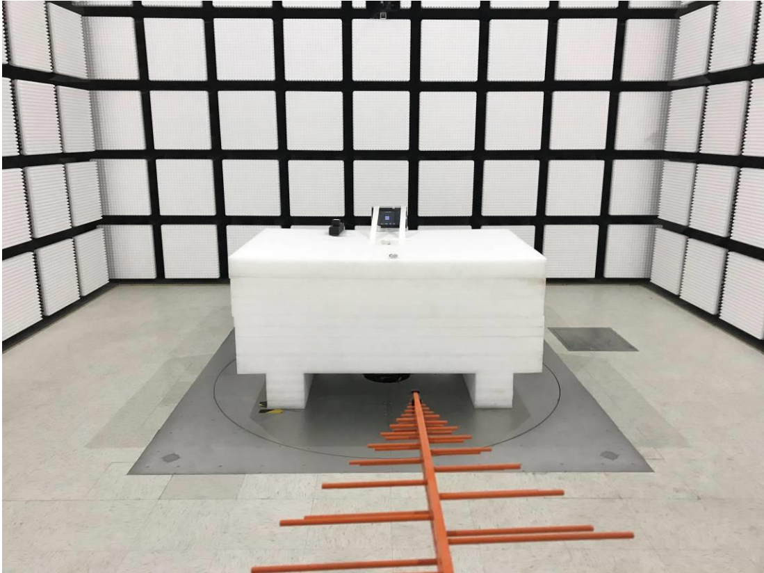
Radiated Emission Below 1G View Adapter
