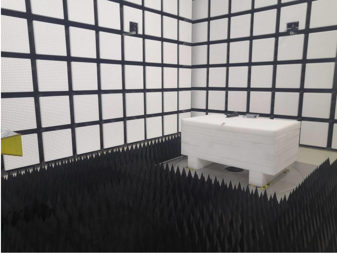
Radiated Emission Above 1G View Adapter
