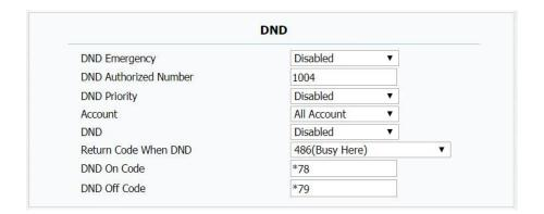
**DND Off Code**: The Code used to turn off DND on server's side, if configured, IT82A(869) will send a SIP message to server to turn off DND on server side if you press DND when DND is on.
