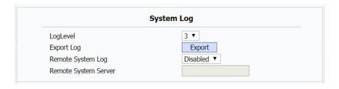
**Remote System Log**: To enable or disable Remote System Log.
