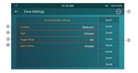
⑥ Configure the status of alarm feature, including disabled, enabled and 24H.
