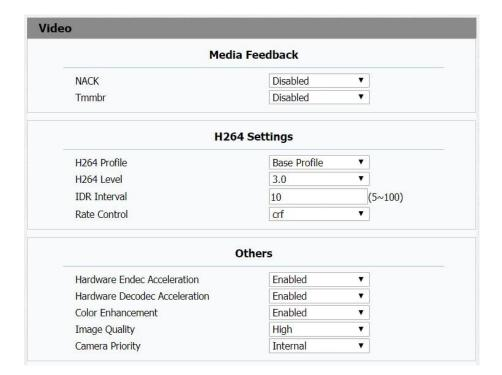
**IDR Interval**: IDR means Instantaneous Decoding Refresh. It is used to control the process of coding and decoding.
