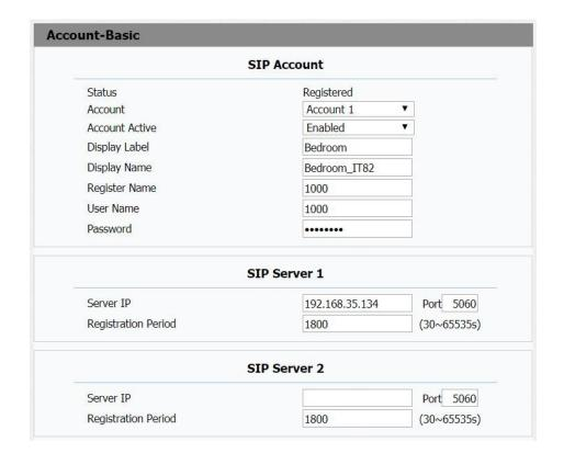
**Register Name**: Allocated by SIP server provider, type in the extension number you want to register.
