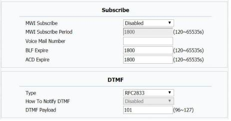
**ACD**: Automatic Call Distribution is often used in offices for customer service, such as call center. The setting here is to negotiate with the server about expire time of ACD subscription.
