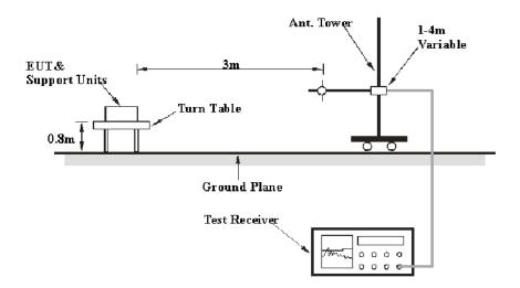
All measurements contained in this report were conducted with ANSI C63.10-2013. The specification used was the FCC Part Subpart C limits.
