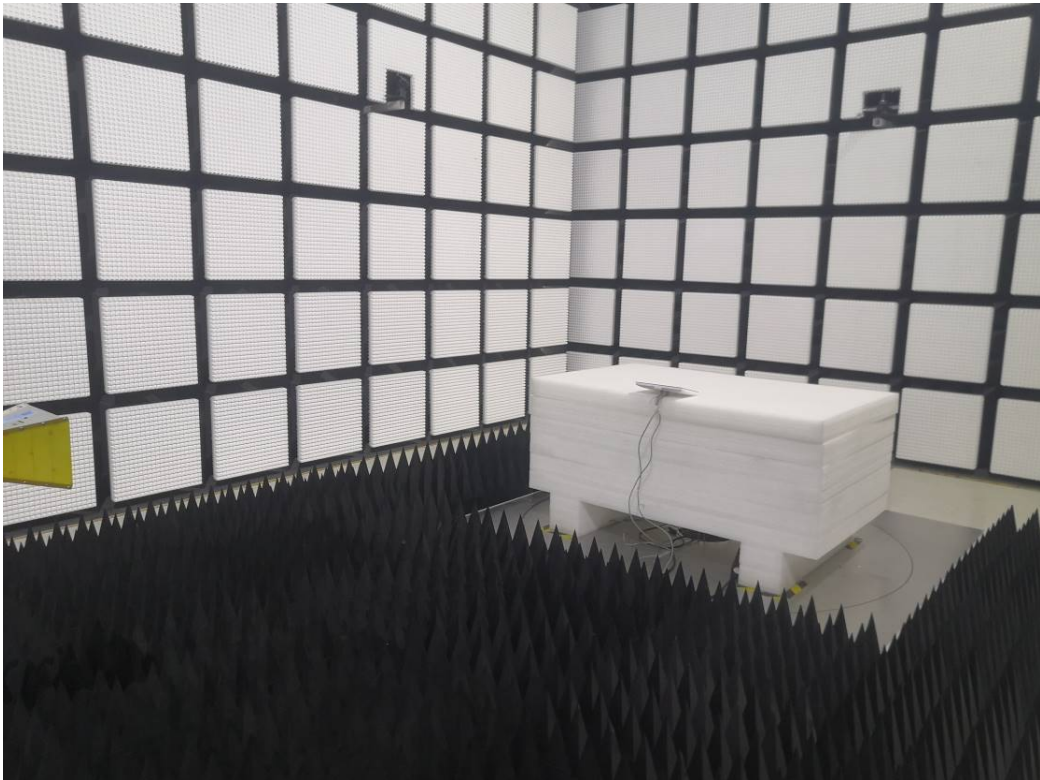
Radiated Emissions Above 1G rear View-PoE
