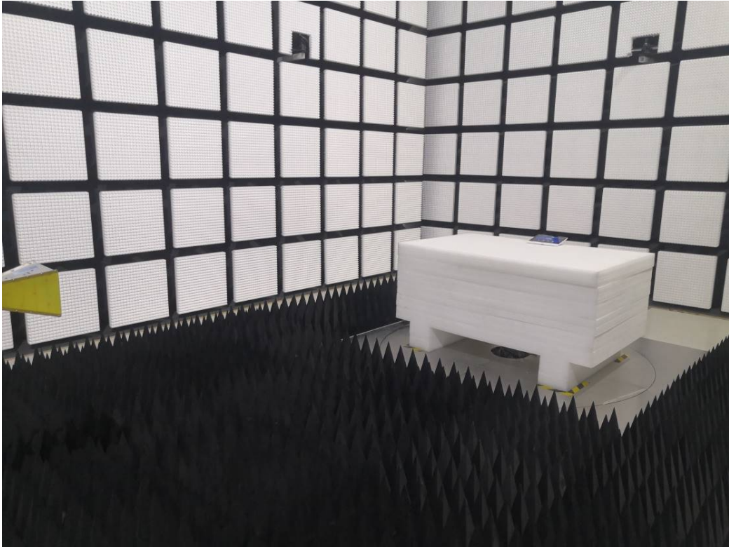
Radiated Emissions Above 1G rear View-PoE
