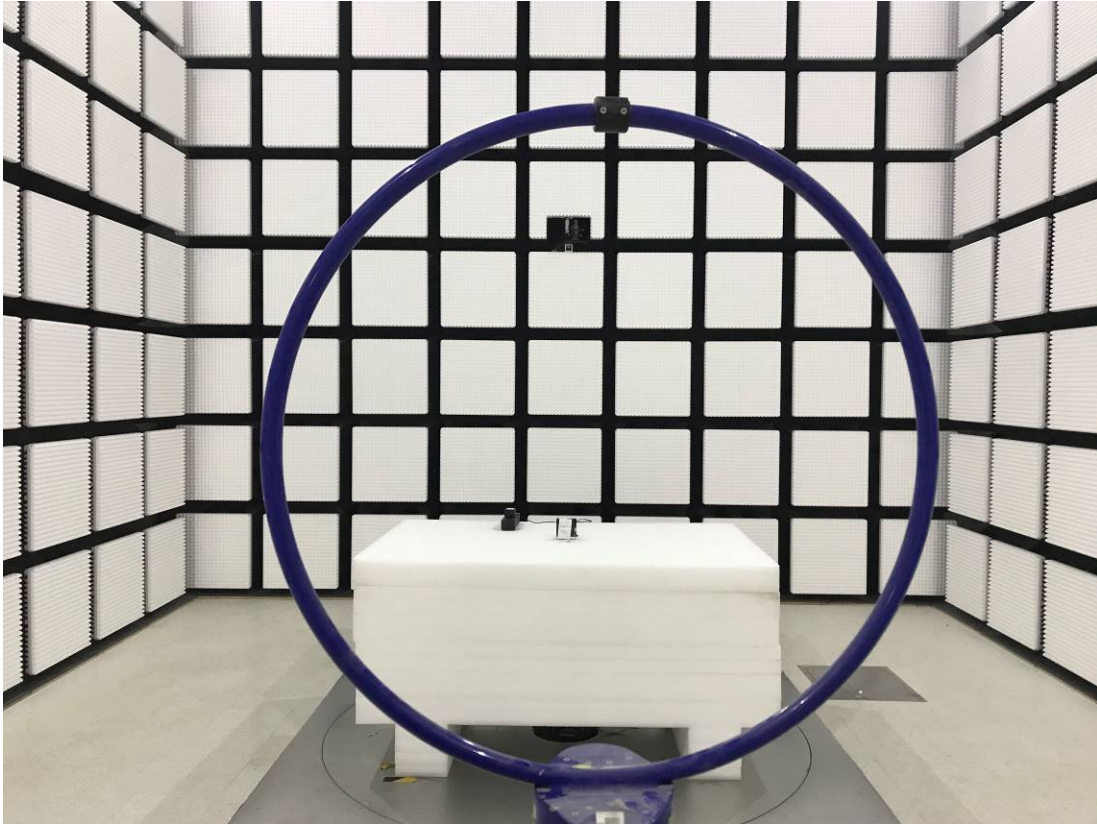
Radiated Emission 30MHz-1GHz Perpendicular View Adapter
