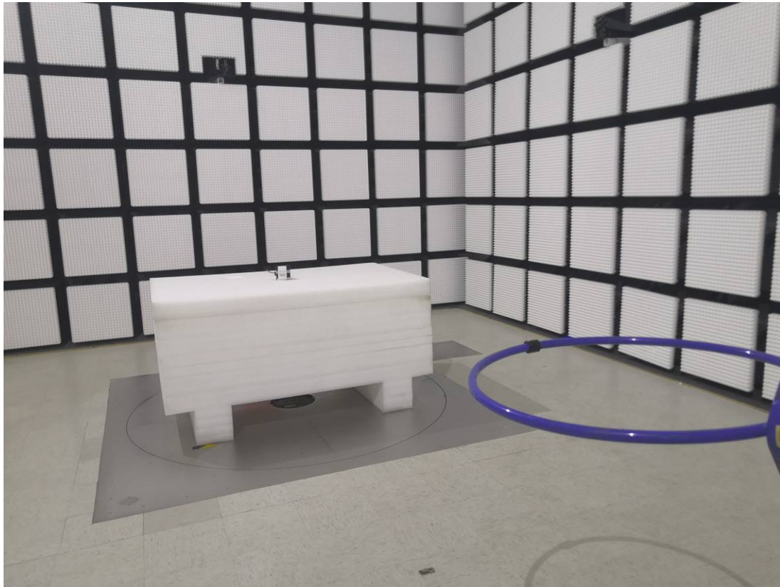
Radiated Emission 30MHz-1GHz View PoE
