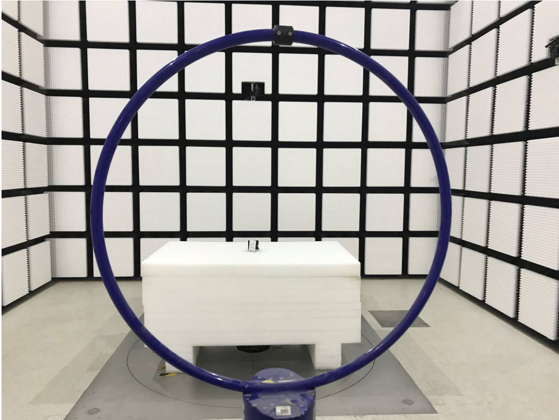
Radiated Emission 30MHz-1GHz Perpendicular View PoE
