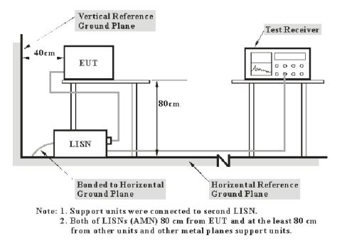
The setup of EUT is according with per ANSI C63.10-2013 measurement procedure. The specification used was with the FCC Part 15.207 limits.
