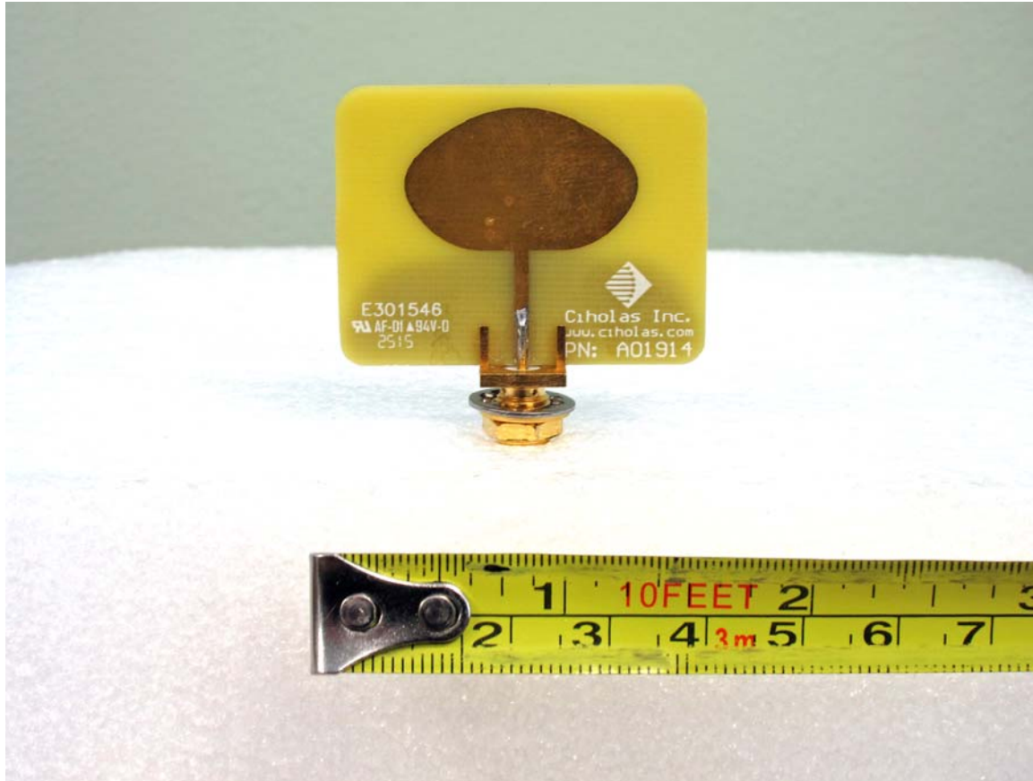
Transmit Antenna Section Antenna Front
