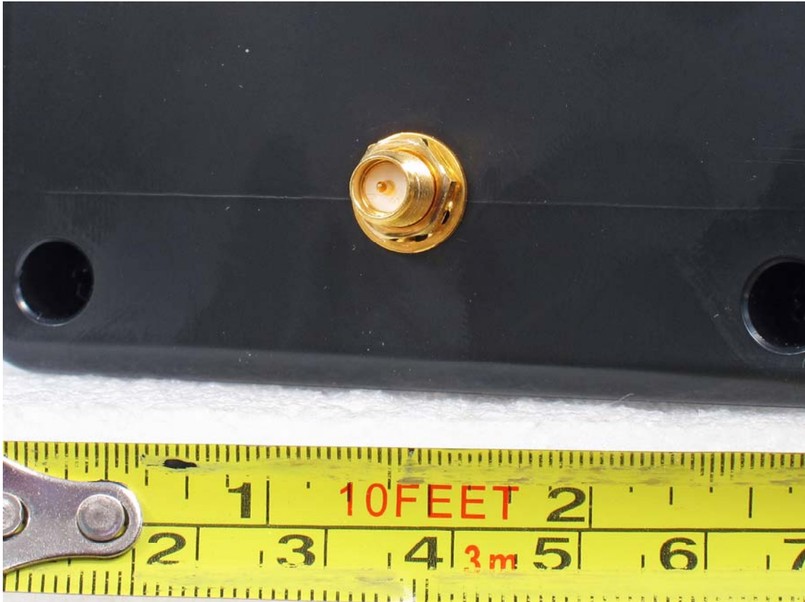
Transmit Antenna Section – Connector Profile
