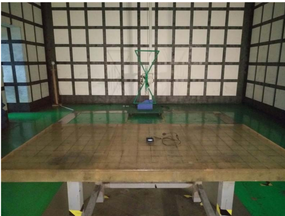
Photograph 2: Radiated Emission Test Configuration, (Below 1GHz) Back
