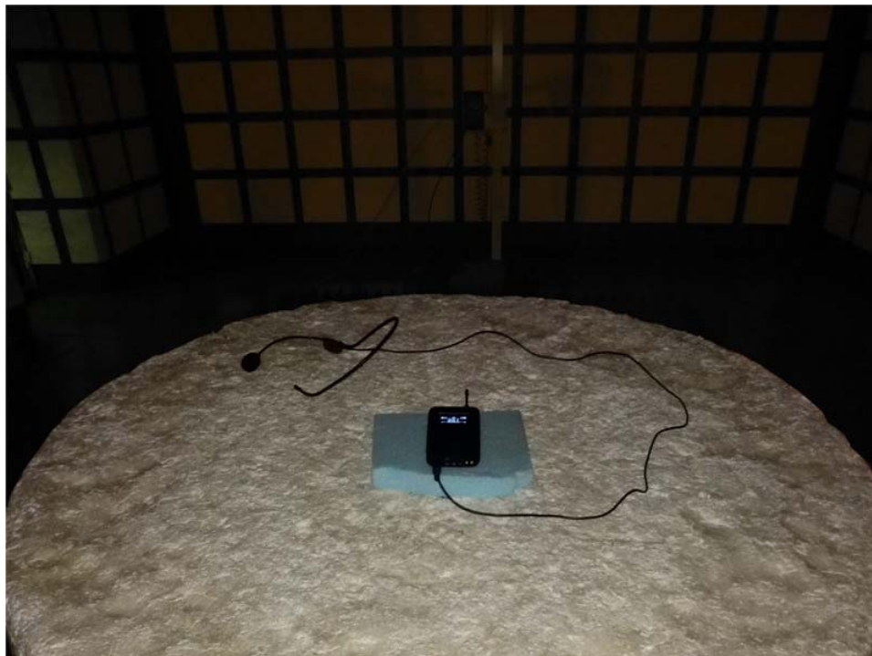
Photograph 3: Radiated Emission Test Configuration, (Above 1GHz) Front
