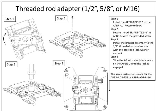
The threaded rod adapter attaches to a rod that is either 1/2"-13, 5/8"-11, or M16-2.
