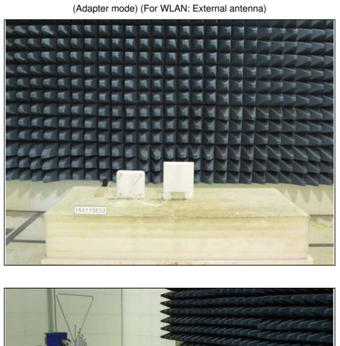
Radiated Emissions below 1 GHz Test
