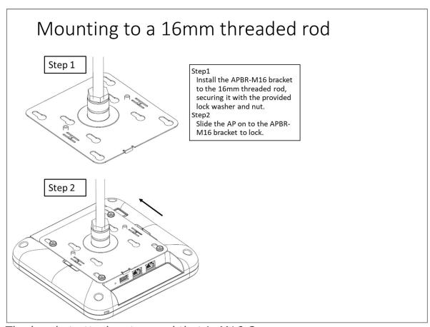
The bracket attaches to a rod that is M16-2.
