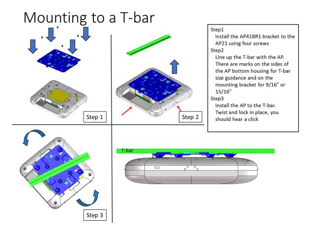
When mounting to a T-bar, please use the screws that are provided which have a head diameter of 8mm and a length of 6mm.
