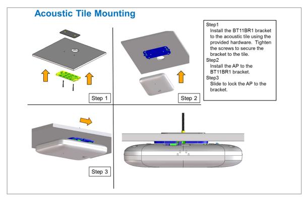
When mounting to an acoustic ceiling tile, please use the screws that are provided which have a head diameter of 7mm and a length of 40mm.
