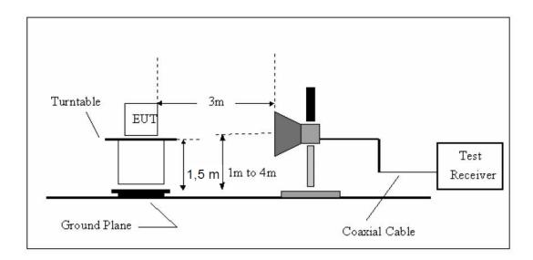
Above 1GHz Test Setup
