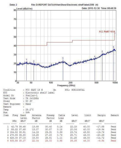
Remark: Level = Read Level + Antenna Factor - Preamp Factor + Cable Loss
