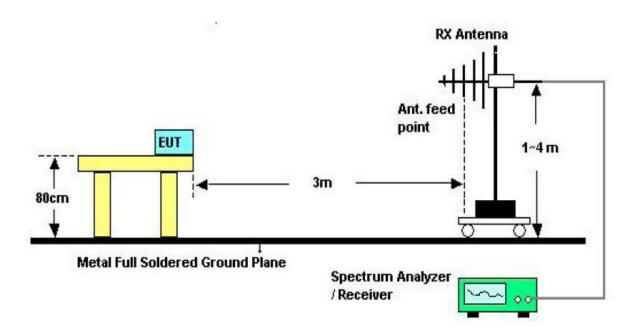
Above 30MHz Test Setup
