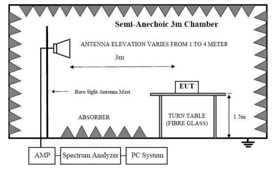
In Semi Anechoic Chamber (3m) Test Setup Diagram for Above 1GHz
