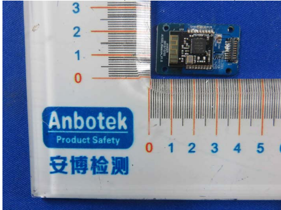
Figure 24 PCB of The EUT-Front View (Bluetooth N51822 iBeacon)
