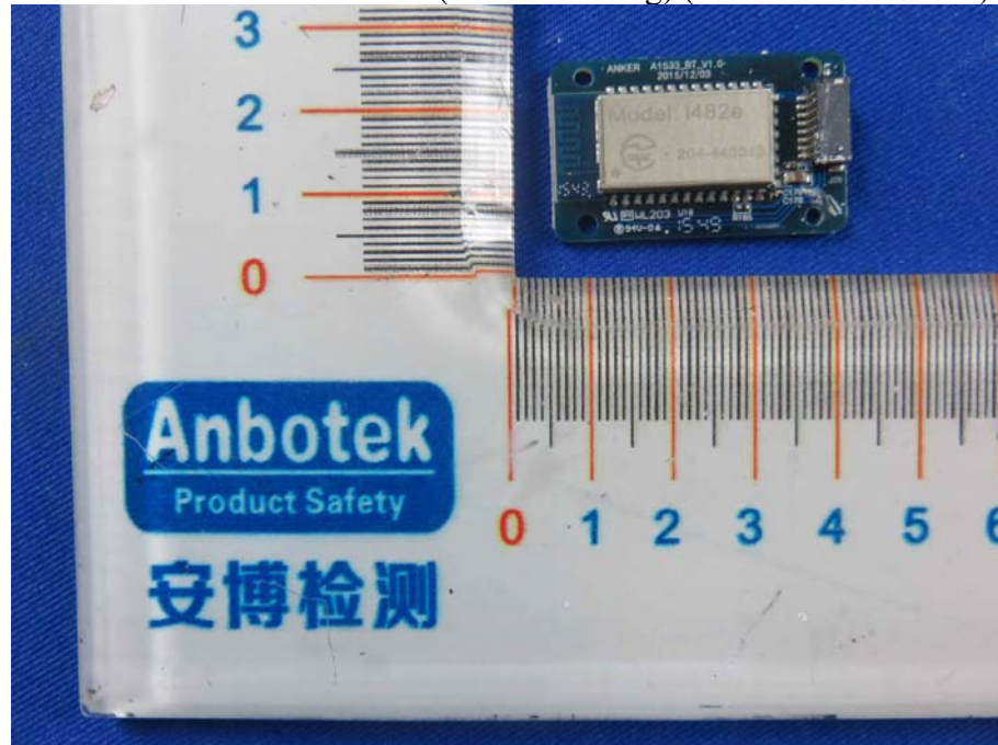
Figure 26 PCB of The EUT-Front View (With Shielding) (Bluetooth CSR8811)
