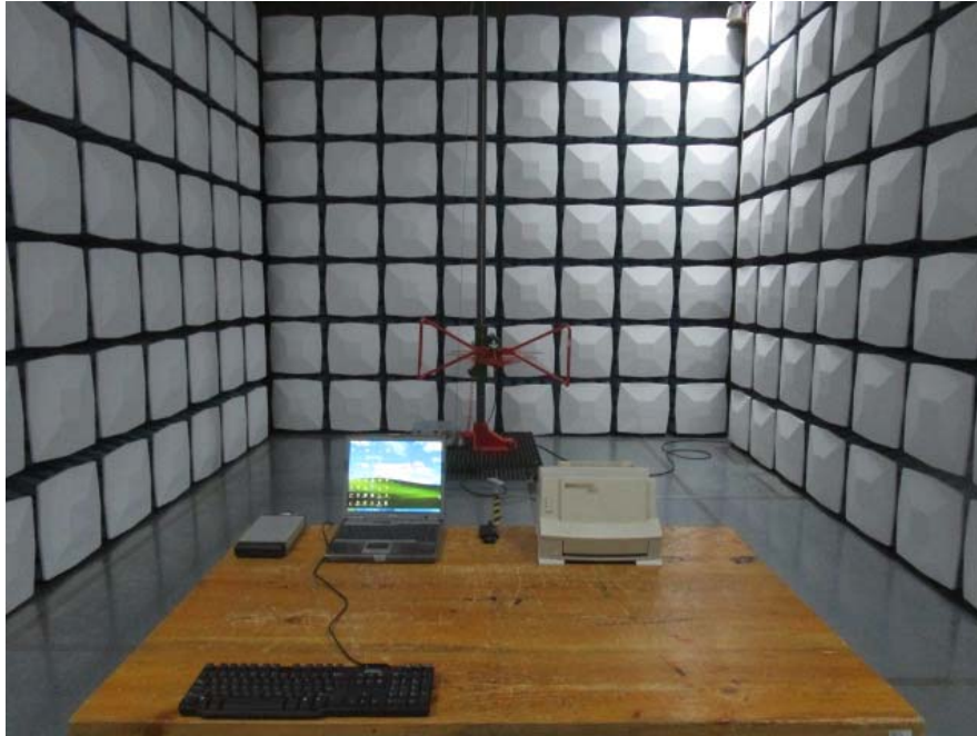
Radiated Emissions –Front View (Below 1GHz)
