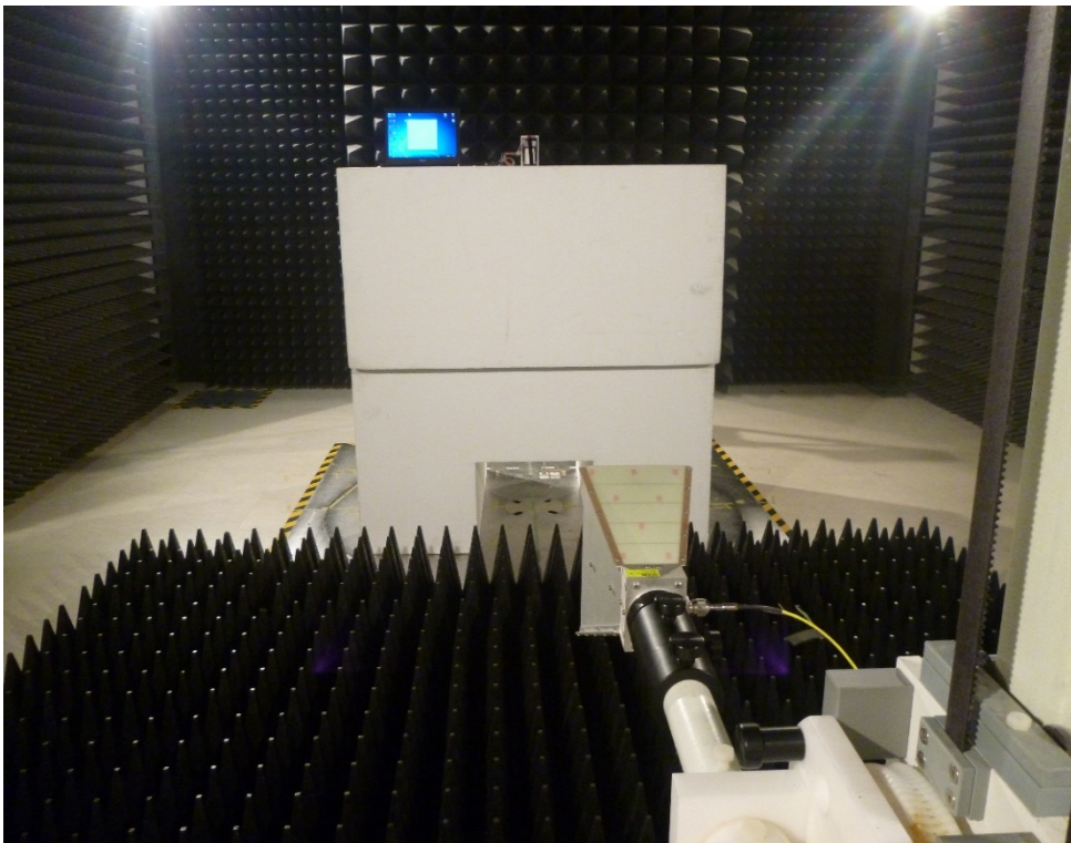
Radiated Emission -Rear View (Above 1GHz)
