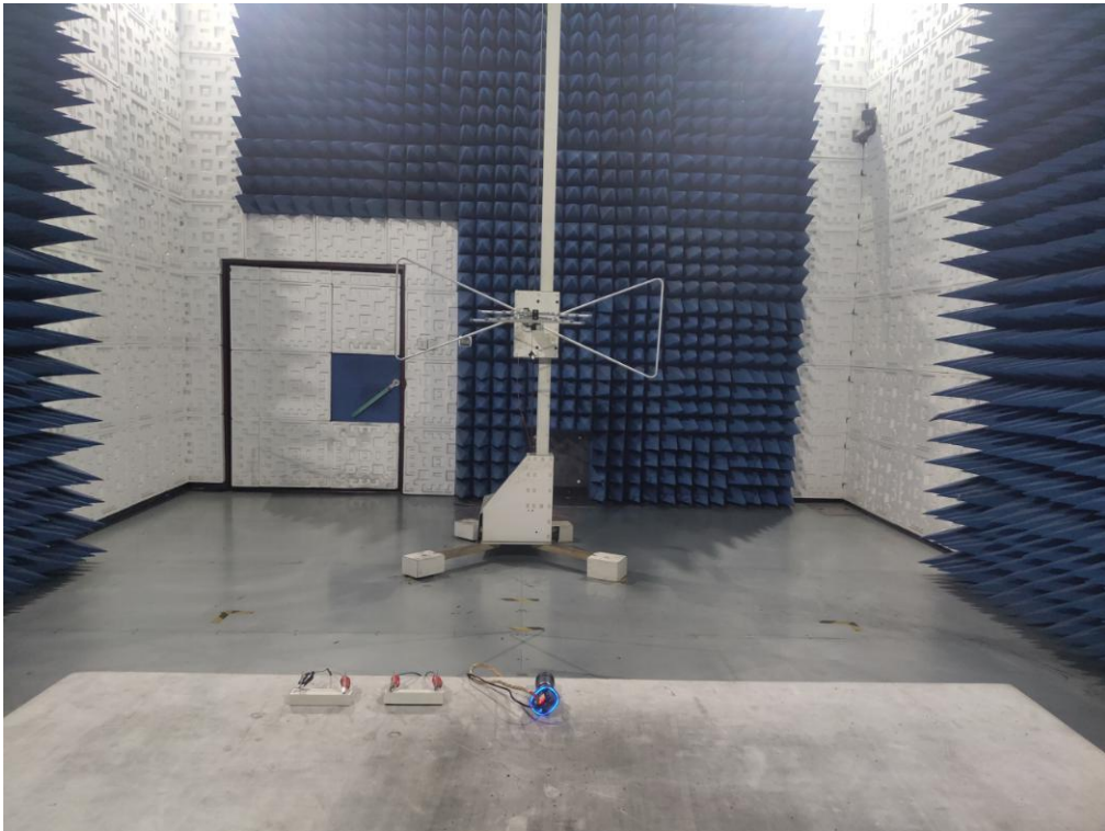
RADIATED EMISSION TEST SETUP ABOVE 1G
