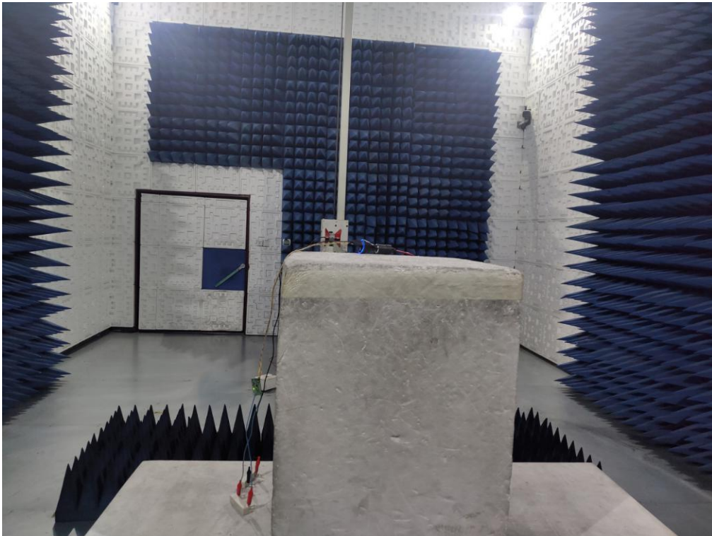
RADIATED EMISSION TEST SETUP ABOVE 1G
