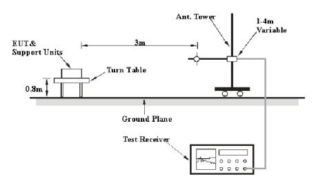
The radiated emission tests were performed in the 3-meter chamber test site, using the setup accordance with the ANSI C63.10-2013. The specification used was the FCC 15.209 limits.
