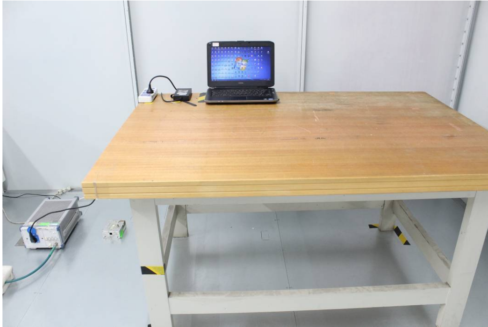
Conducted Emission Front View (Below 1 GHz)
