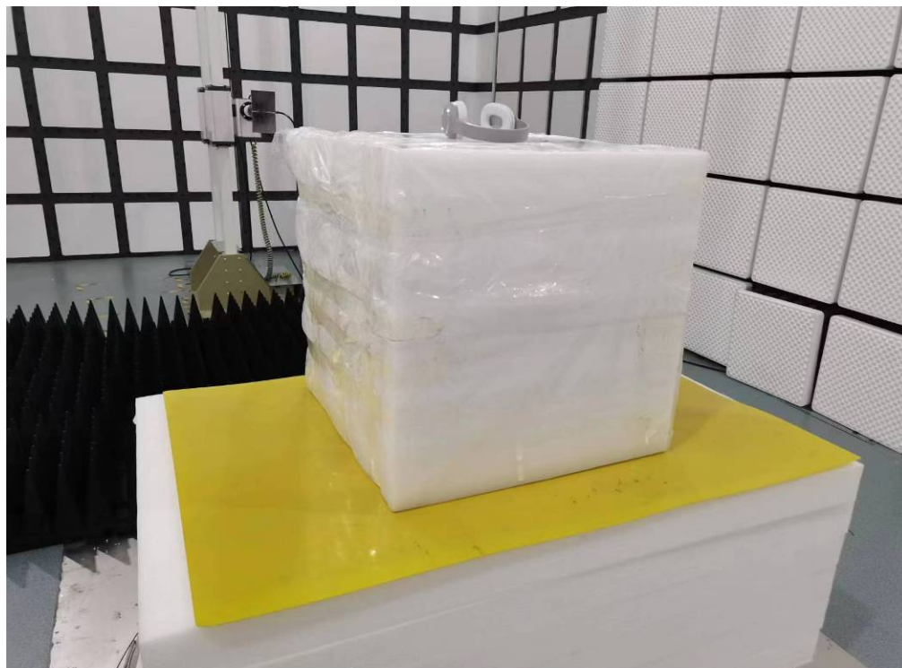
Photo of Radiated Emission Measurement (Above 1G)
