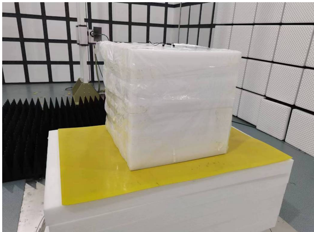
Photo of Radiated Emission Measurement (Above 1G)
