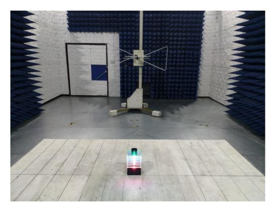
RADIATED EMISSION TEST SETUP ABOVE 1GHZ
