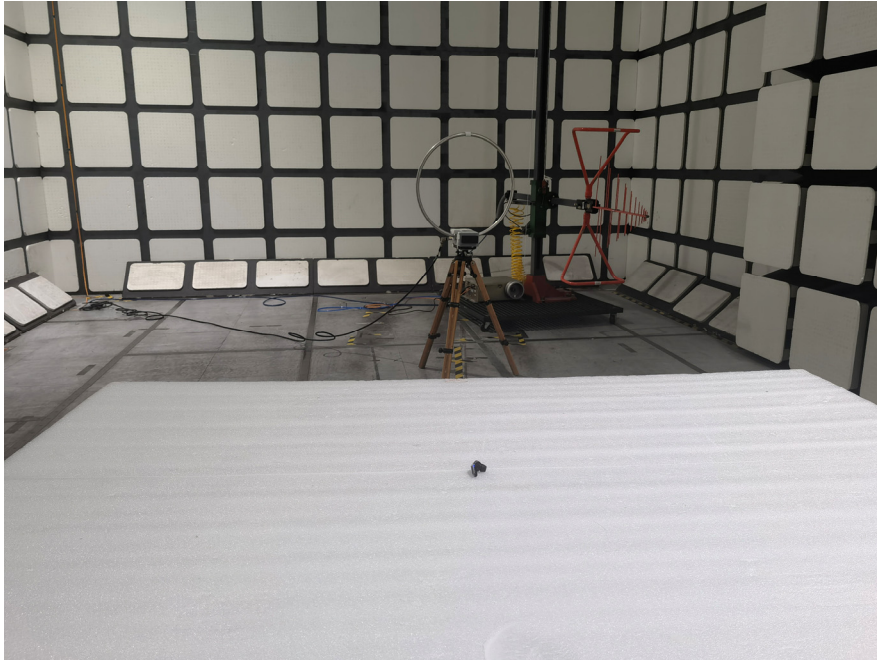
Radiated Emissions View (9 kHz- 30 MHz)
