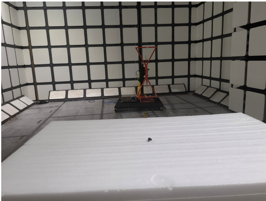
Radiated Emissions View (30 MHz- 1 GHz)
