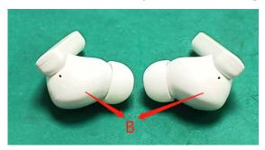
Conclusion: Based on the above description of area A to B, we conclude that the device is unquestionably too small for enabling the FCC certification No. to be printed onto any surface. We therefore request to move the FCC certification No. to the user's manual and charging case.
