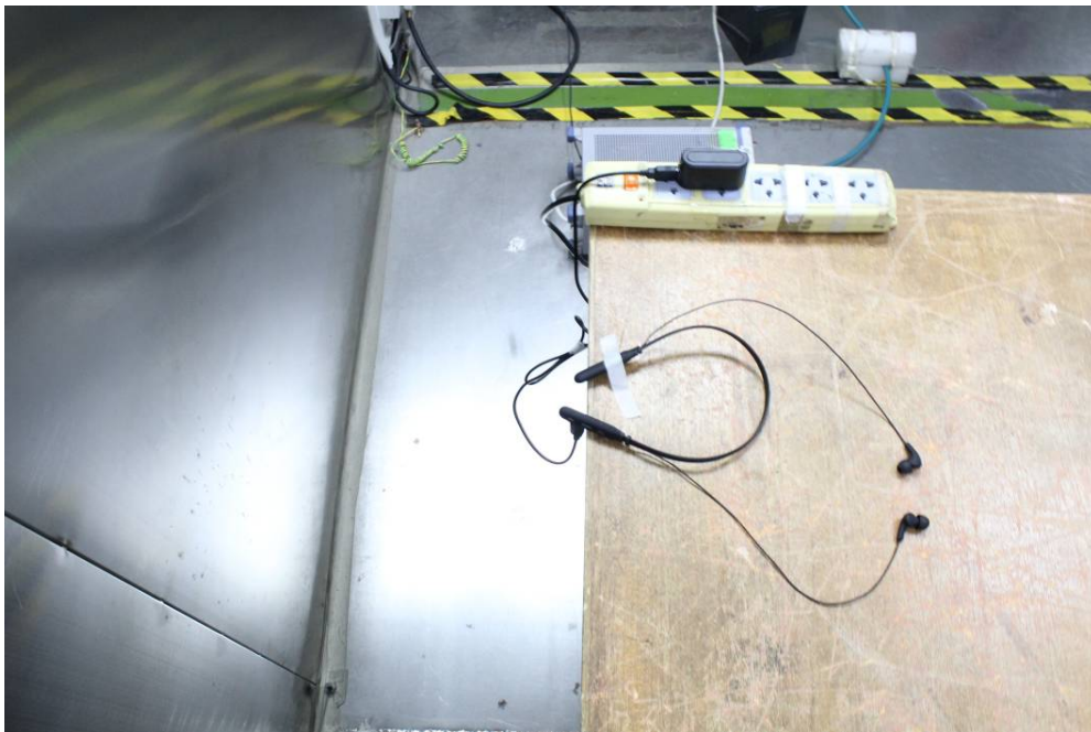
Conducted Emissions - Side View
