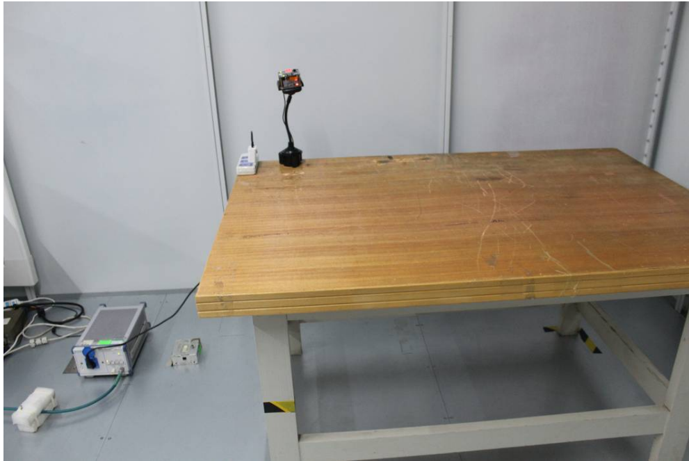
Conducted Emissions - Side View
