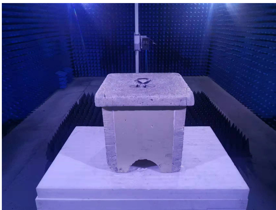
Photo of Radiated Emission Measurement (Above 1G)
