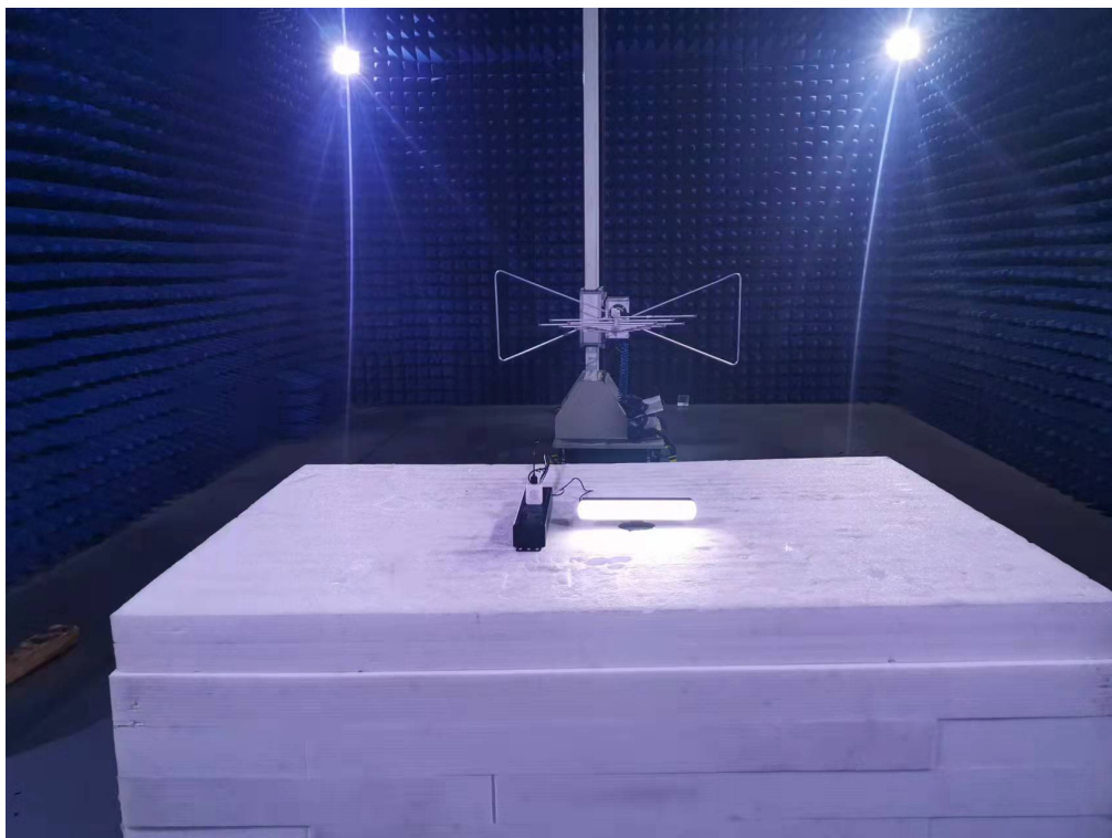
Photo of Radiated Emission Measurement (Above 1G)
