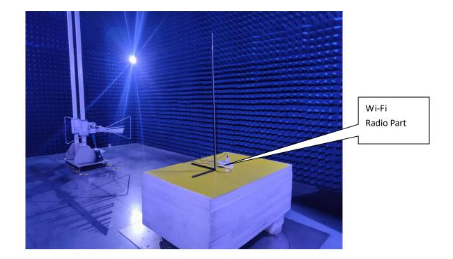
Photo of Radiated Emission Measurement (Above 1G)
