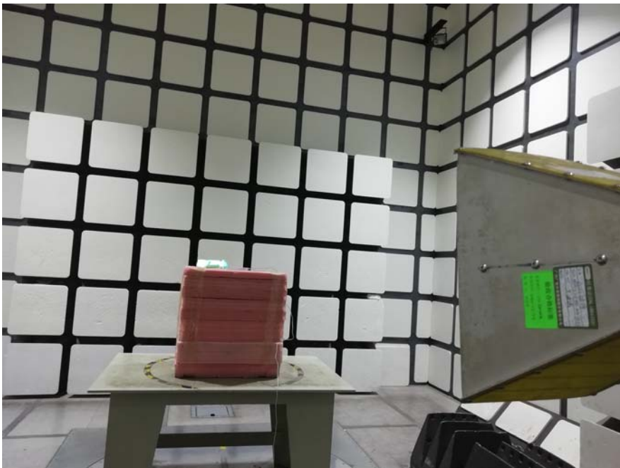
Radiated Emissions View (Above 1 GHz)
