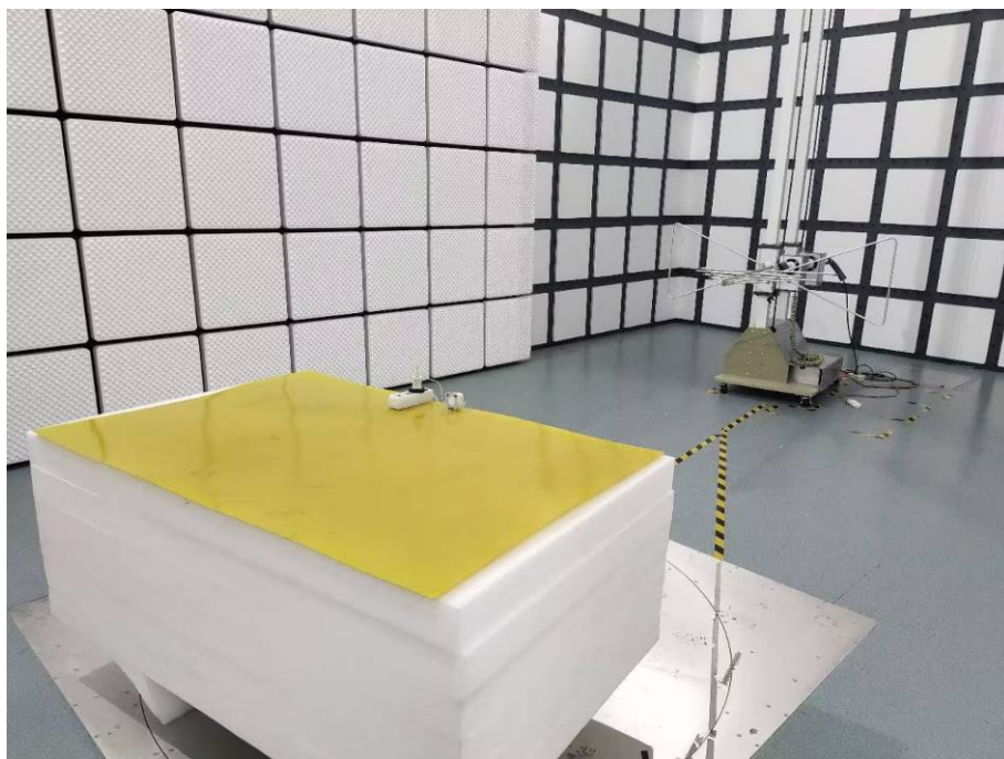
Photo of Radiated Emission Measurement (Above 1G)
