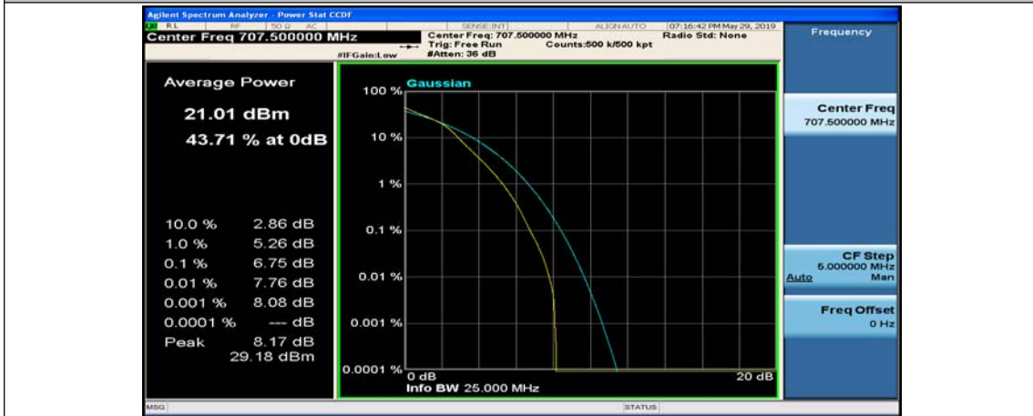
(Channel Bandwidth: 5 MHz)_MCH_16QAM_12RB#13
