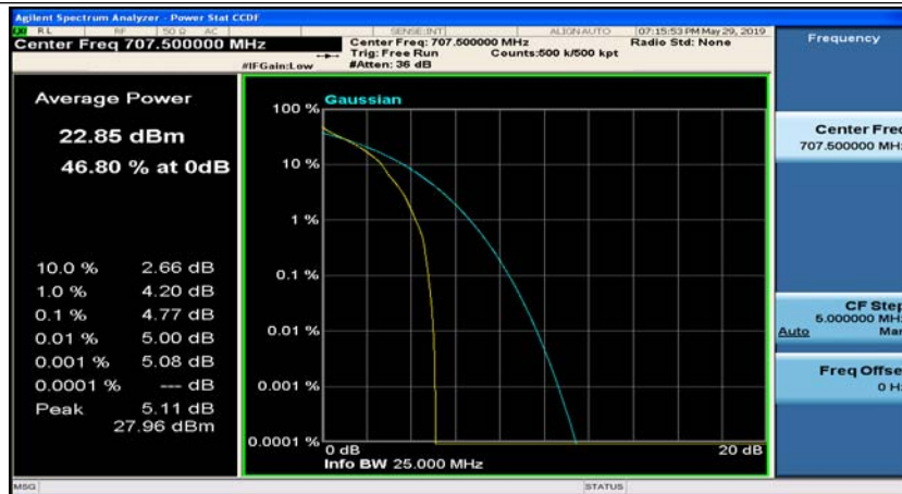
(Channel Bandwidth: 5 MHz)_MCH_QPSK_12RB#0
