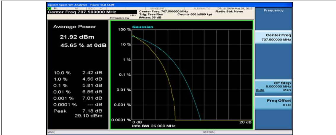
(Channel Bandwidth: 5 MHz)_MCH_QPSK_25RB#0
