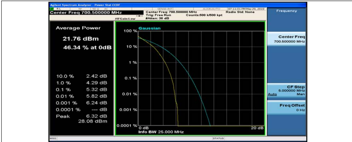
(Channel Bandwidth: 3 MHz)_MCH_QPSK_1RB#0
