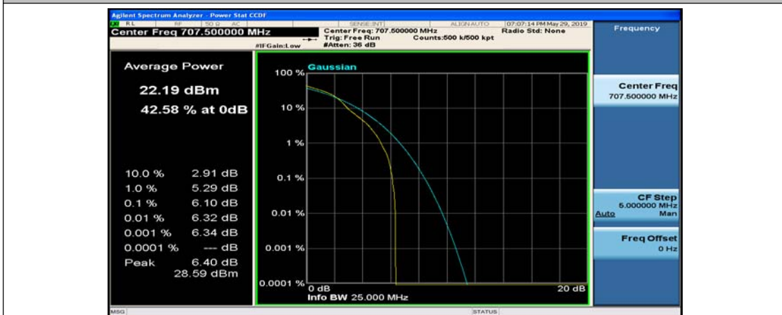
(Channel Bandwidth: 1.4 MHz)_MCH_16QAM_1RB#5
