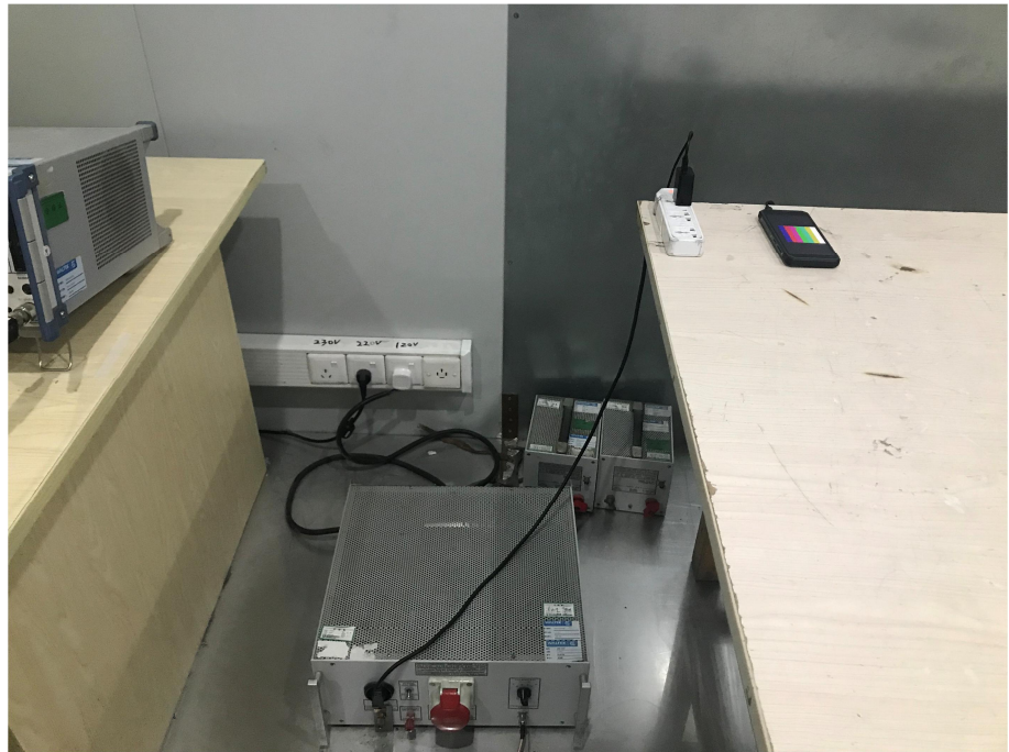
Conducted Emission Test Setup
