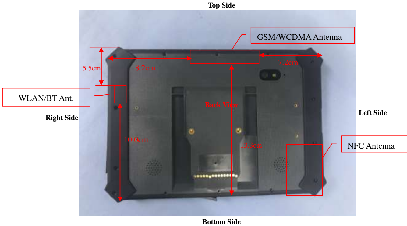
Block Diagram for EUT Antenna Position
