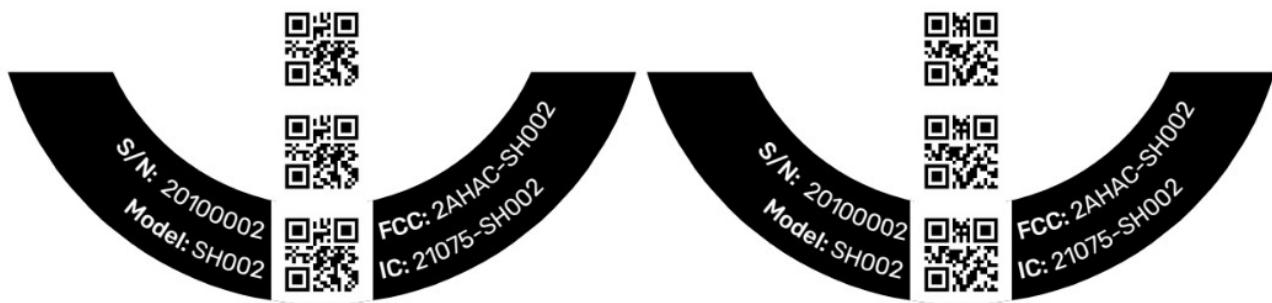
Two labels using successive serial numbers side by side. The two top QR codes are used during manufacturing only and do not appear on the final product. Size in document is not to scale, see below for dimensions.
