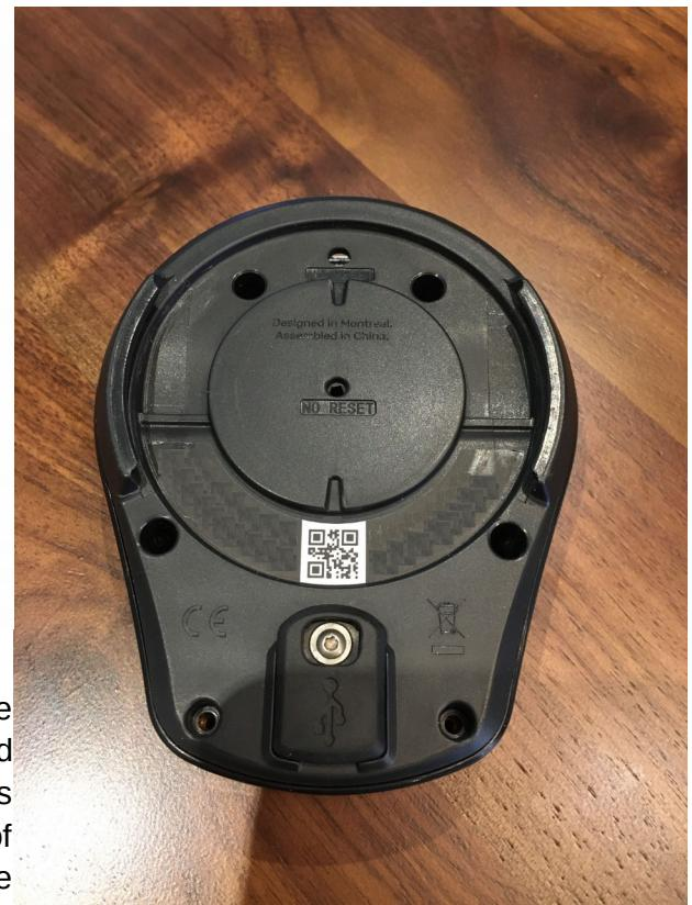
In the picture to the right, a prototype label can be seen on the bottom of the plastics casing as used during the NPI phase of the product design. This is not a final label, but rather used as a an example of location on the bottom of the plastic casing. See below for label specifications
