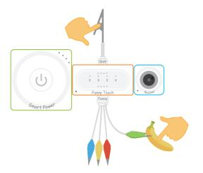
After the Funny Touch is connected to the buzzer, you can touch Funny Switches of different colors or touch several Funny Switches at the same time. Listen, the buzzer is making different sounds!
