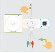
Use a Funny Switch to clip on a conductive object, such as a banana. Touch the banana with one hand and the metal part of the GND wire clip with another hand. See what will happen!
