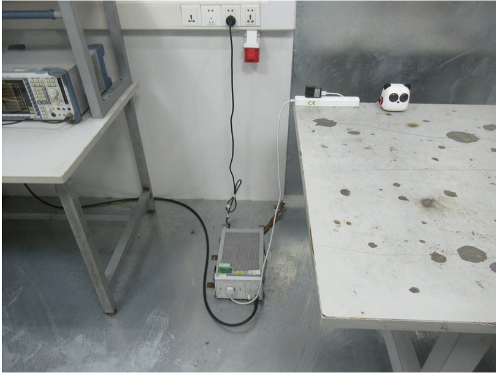
Photo of Conducted Emission Measurement
