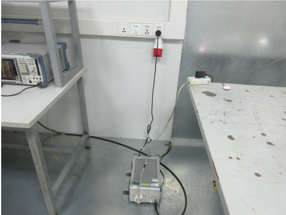
Photo of Conducted Emission Measurement
