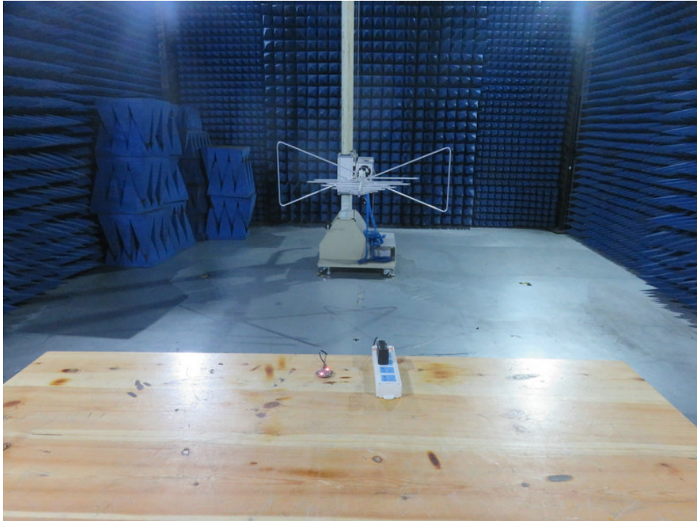
Photo of Radiation Emission Test
