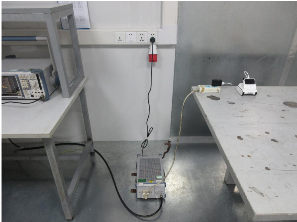
Photo of Conducted Emission Measurement
