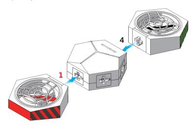
After connecting power modules to the master controller module, fit the master controller module onto the hovercraft hull.
