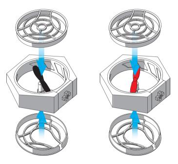
After fitting the protective covers, attach the 4 power modules onto master controller module according to the directions in diagram below. Check that the protective covers are fitted in the accurate places and that the power modules are attached securely to the master controller module.
