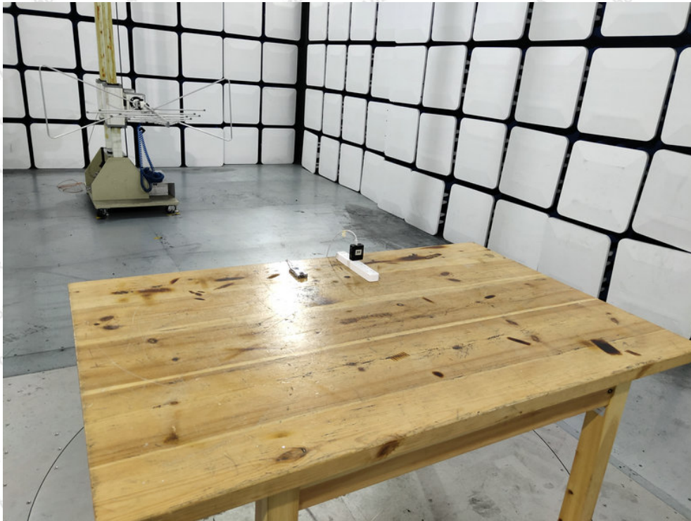
Photo of Radiation Emission Test
