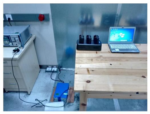
FCC RADIATED EMISSION TEST SETUP BELOW 1GHZ
