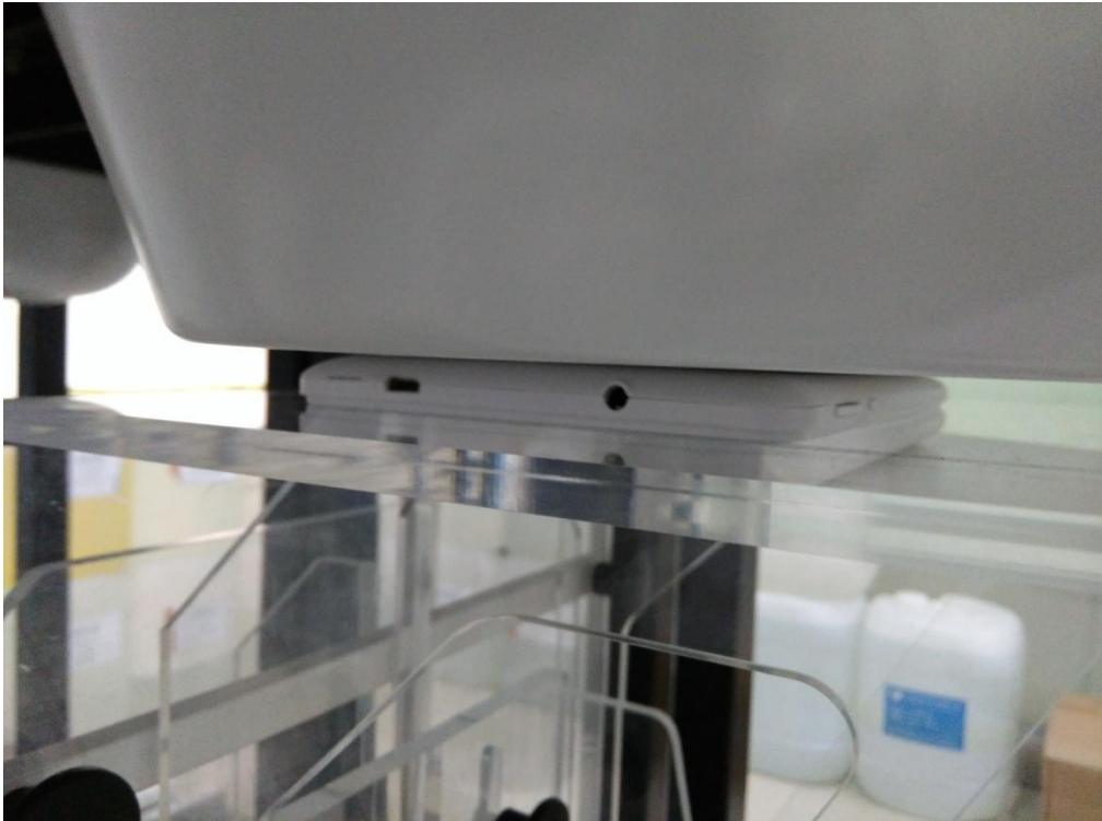
Body Back side(separation distance is 0mm)
