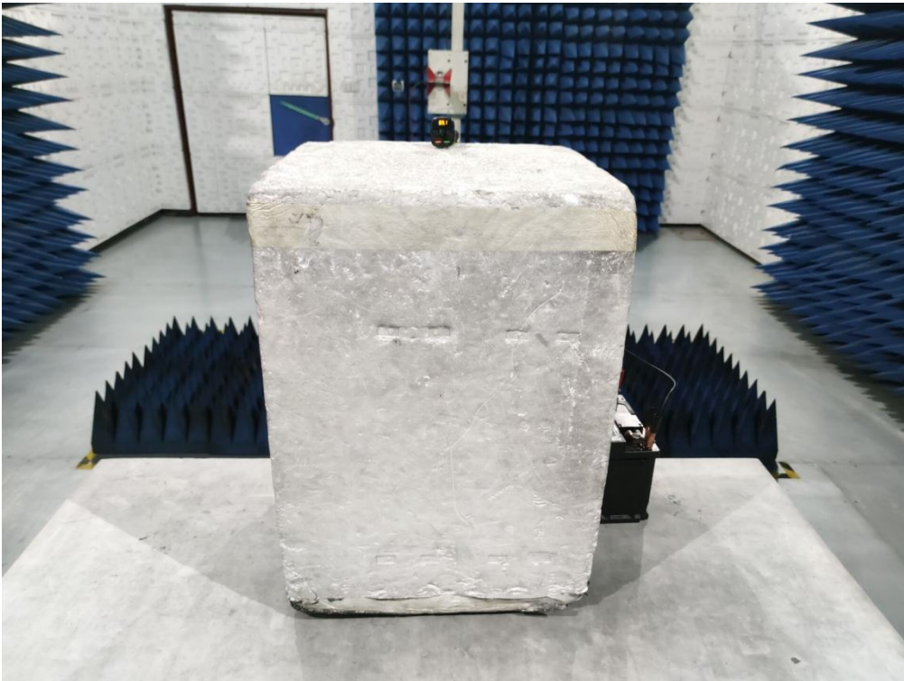
RADIATED EMISSION TEST SETUP ABOVE 1GHz
