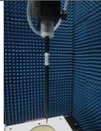
Fig.8.2 Photo of E-Field Probe
