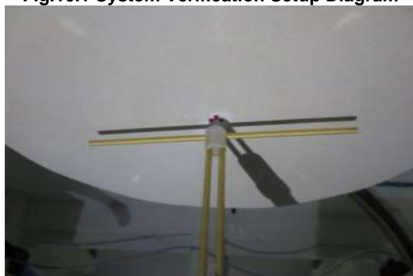
Fig.10.2 Photo of Dipole setup
