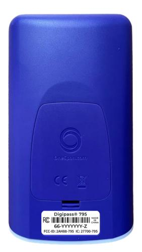
Serial number of the device and regulatory identifiers are on a label at the back of the device.
