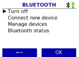
When connecting to a new computer for the first-time using Bluetooth, the device needs to be paired with that computer. This can be done by selecting 'Connect new device'. That will put the authenticator device into pairing mode and make it visible for other devices for 30 seconds. From your computer's Bluetooth settings, select new device and from the list of devices pick DP795.
