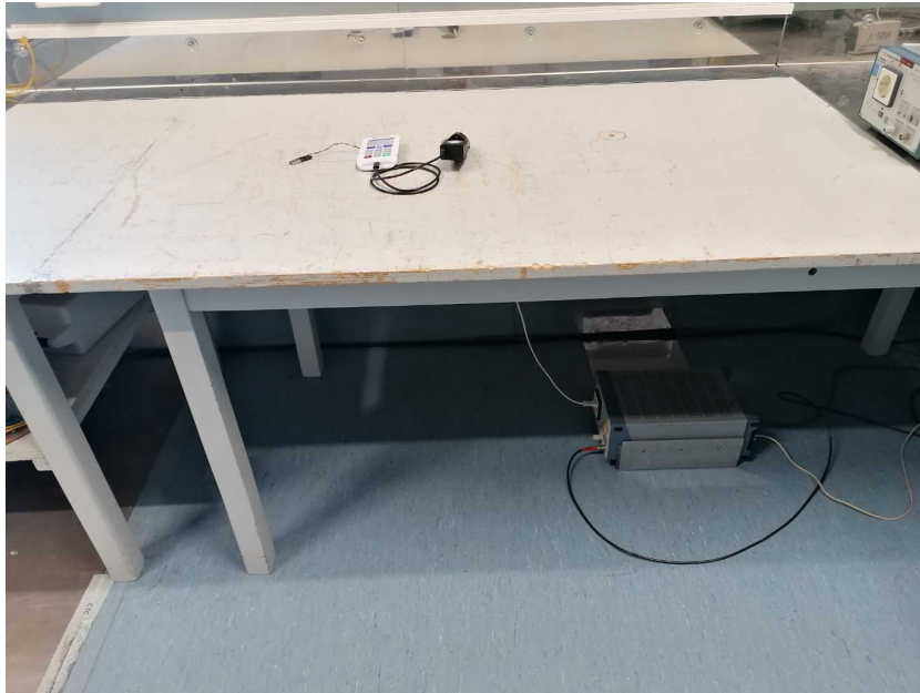
Photo 11: AC conducted emission test setup
